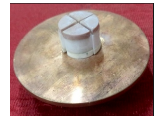
MEMS DRA with Wideband and High Gain capability
